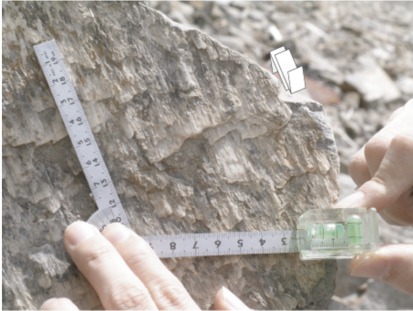
Slickenside lineation on a fault plane in a Cretaceous formation, Wakayama, Japan.
